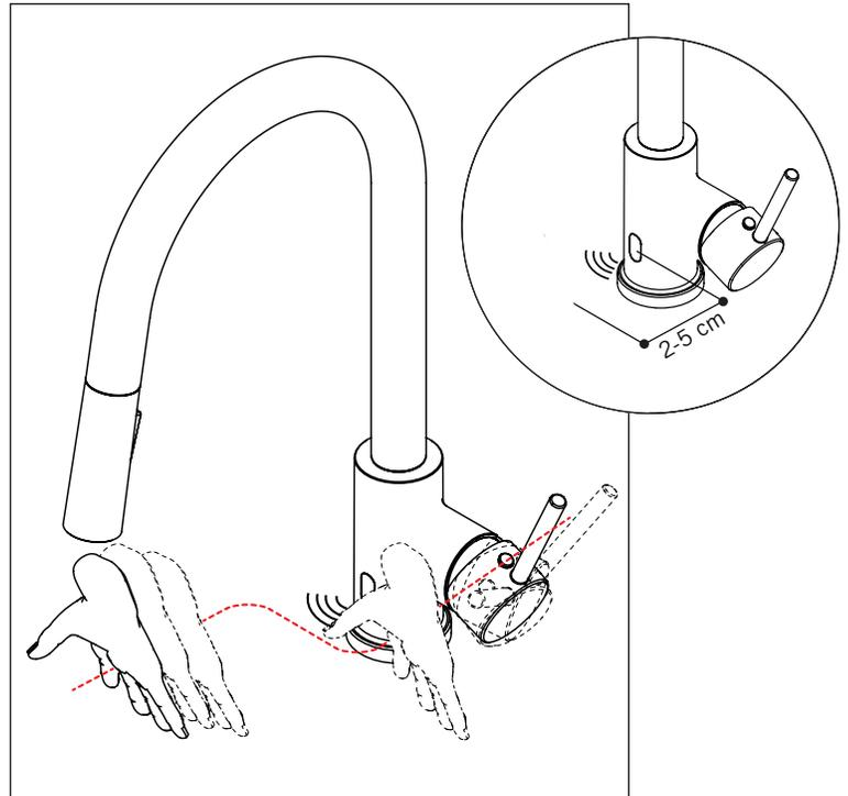
\*The solenoid valve was designed to hold against line pressure 24/7. It is the line pressure that turns-it off and it requires power to turn on, therefore the faucet cannot turn on by itself.
